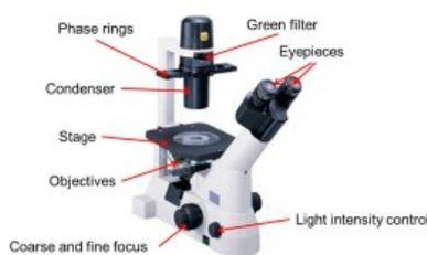
A typical inverted phase contrast microscope - Nikon TS100
